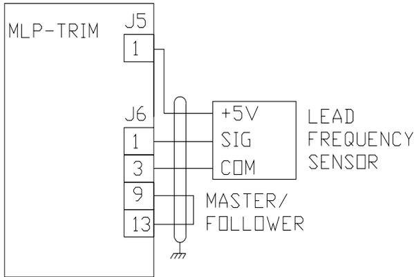
2. Enter the pulses-per-revolution of the lead (master) sensor into CP-30 (PPR Lead).
