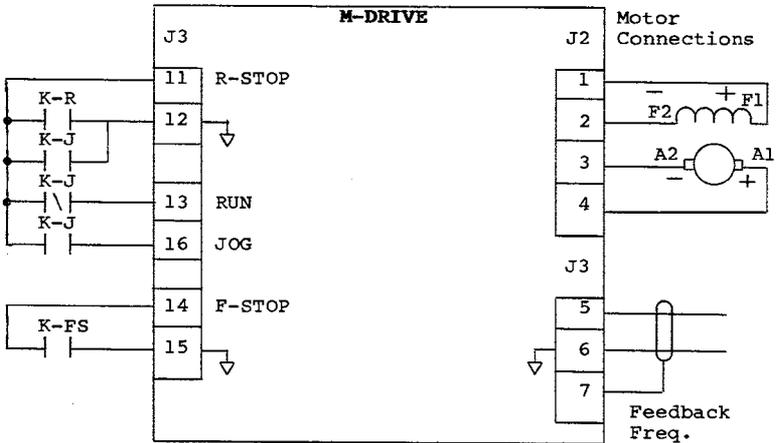
Figure G-2: Relay Start & Stop Wiring Connections
