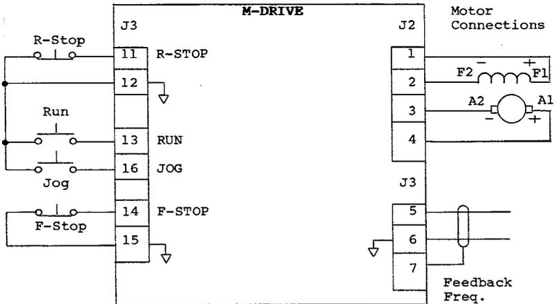
Figure G-1: M-Drive Wiring Connections without Relays
