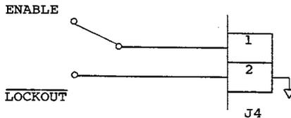
Figure 3-18: Keypad Lockout
