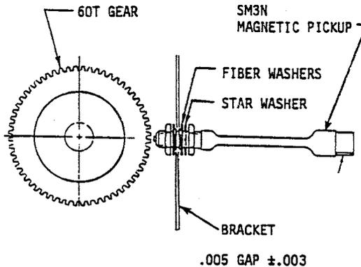
\*Installed to insulate pickup
