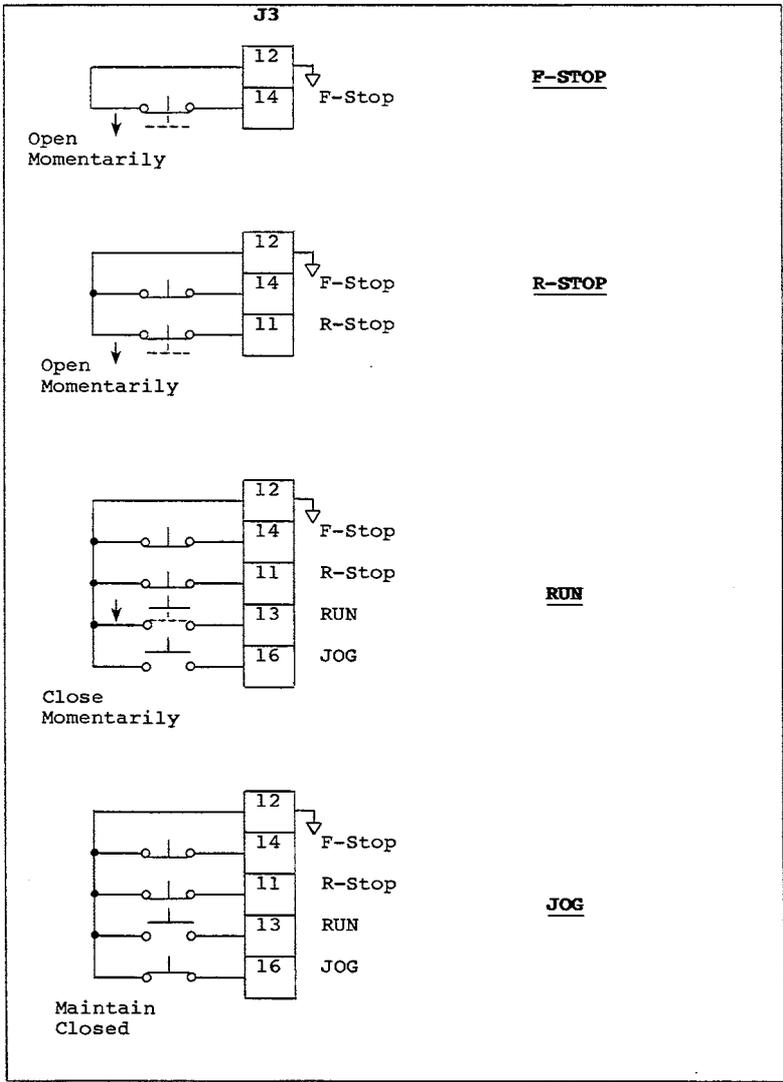
Figure 1-7: Run/Stop Logic
