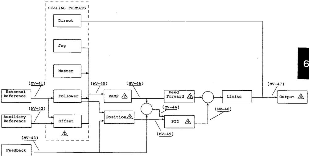
Figure 6-1: M-Drive Operation Function Block Diagram
